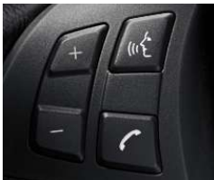
□ Voice control system: for adjusting the radio station, navigation routes etc. while driving. Functions are shown on the Control Display at the same time (this feature is included in the Navigation system Professional**).
