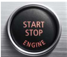
■ Start/Stop button for starting the engine. After inserting the ignition key you can start or stop the engine by pressing the button.
