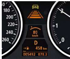
□ Active Cruise Control with Stop & Go function actively maintains a pre-selected speed and following distance to the vehicle in front – with automatic restart for driving in typical stop-and-go situations such as slow moving traffic.
