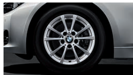
□ 16" light-alloy wheels V-spoke 390, 7 J x 16, 205/60 R 16 tyres (standard on 320i and 318d).
