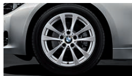
□ 17" light-alloy wheels V-spoke 395 with mixed tyres, 7.5 J x 17, 225/50 R 17 tyres at the front, 8.5 J x 17, 255/45 R 17 tyres at the rear.
