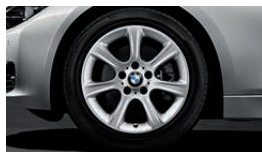
□ 17" light-alloy wheels star spoke 394, 7.5 J x 17, 225/50 R 17 tyres (standard on 328i and 335i).
