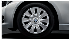
■ 16" steel wheels with full wheel covers, 7 J x 16, 205/60 R 16 tyres (standard on 316d and 318d).
