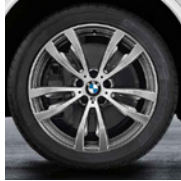
Stils 469M Priekš. 275/40R20 106V Pirelli Ice Zero r-f RFT RDC i R 36112456160
